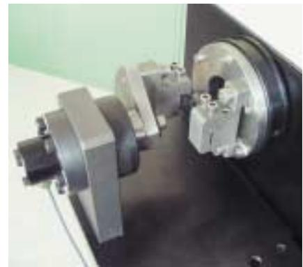
Gripping head for sheet metal tests
